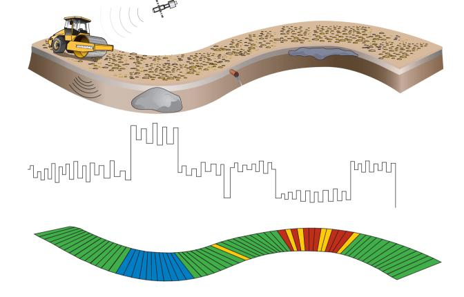
Continous Compaction Control using accelerometer based on stiffness readings allows the roller operator to "see" below the surface.
