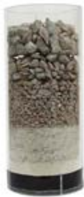
Figure 1. Constituents of a typical asphalt mix. The black part in the bottom represents the volume fraction of the binder.
