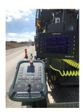
Thanks to the quality system the paving workflow can be optimized because it documents how many kilograms you have put down per square meter paved and registers instances of stop, start and loading to document it. This enables a better self-control which is supported by the analyzing and reporting functions of the tool. The collected data can easily be compared to the required specifications and used for creating job reports. Next
