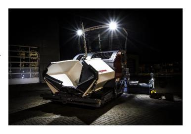
home light guides operators safely up and down the paver. If the machine is shut down, the back lights will continue to shine for one minute so all workers can safely find their way. The integrated side shield lights illuminate the joint and front part of the shields, hence operators have a better visibility.
