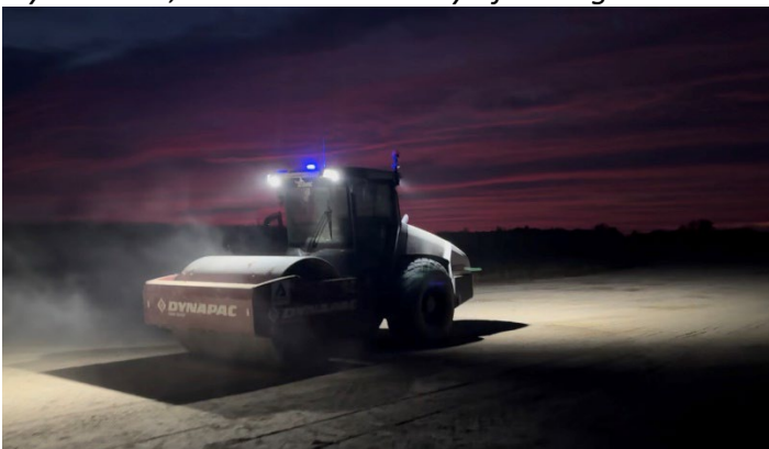
Dynapac CA2500D Seismic Roller equipped with the Bluelight Autonomous Kit at the Scout Plant in Blythewood, SC – Photo courtesy of Bluelight Machines and Landmark Construction.
